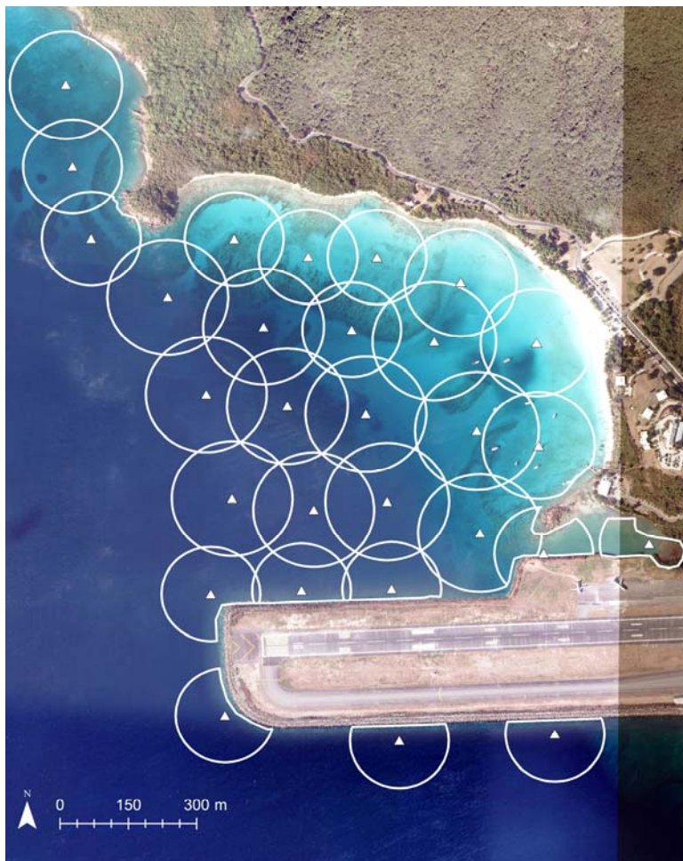
Figure 34. Brewer's Bay, USVI with the entire acoustic array, completed July 2015.
