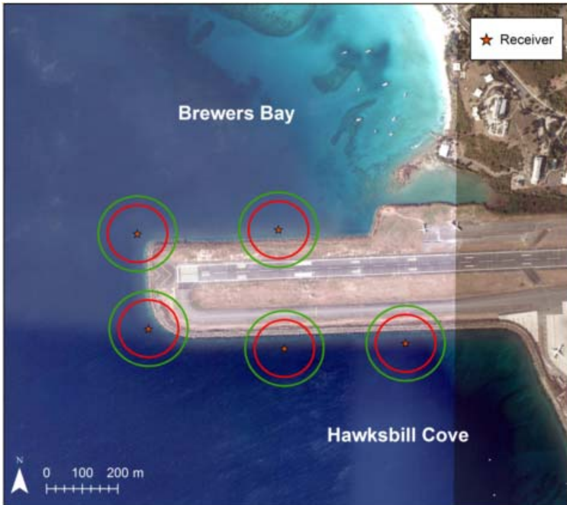
Figure 31. Brewer's Bay map showing the 50% detections range of the receivers using the V16 and V13 acoustic transmitters. The green circles are the detection range for the V16 tags (105m) and the red circles are the detection ranges for the V13 tags (80m).
